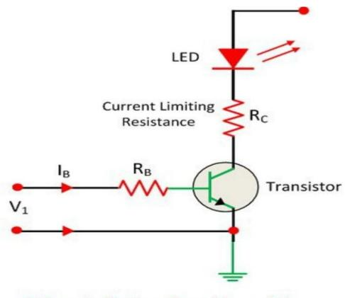
LED controlled by a Transistor switch
