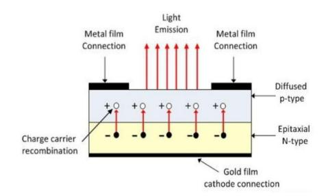
region. This gold layer of cathode helps in reflecting the light to the surface.
